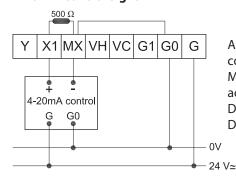
A 500  $\Omega$  resistor must be connected between X1 and MX. (Not delivered with the actuator) Dip switch 2 must be OFF and
